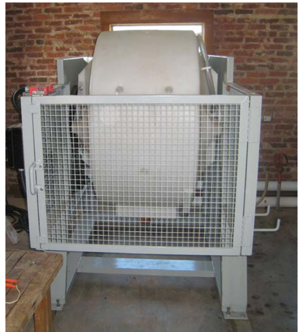
Tanning drum in which all chemical tanning steps are carried out.
