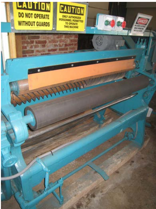
Fleshing machine to remove unwanted tissue from the flesh side of the skin.
